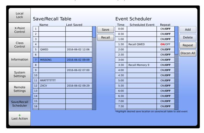
To save or recall a configuration, use the scroll bar on the right hand side to locate the desired numerical memory location. Touch the line item to highlight it, then select the save button to save the configuration or the recall button to recall a saved configuration. In either case, a confirmation window will appear prompting the user to confirm the action.
