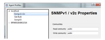
Now you should be back on the Tree tab. Select the bubble option for SNMPv2c:
